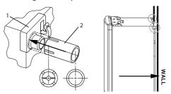
Fig. 1. Push Stopper (2) onto part (1) until the end
