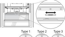
Open state : Move knob to the left(type1) Closed state : Move knob to the right(type3) Recommended state : Middle position(type2)
