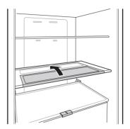
2 Lift the front side of the shelf and shift it under its back side. From this position, both sides of the shelf can be lifted up to free more space.
