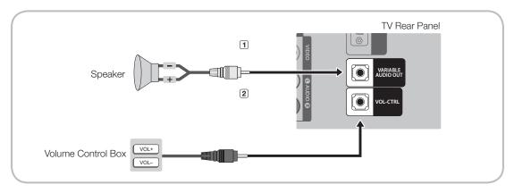
1. Connect the VARIABLE AUDIO OUT port of the TV to the Bathroom Wall Speakers of the hotel.
