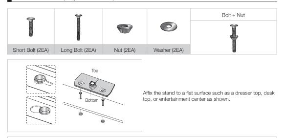
**WARNING**: To prevent injury, this apparatus must be securely attached to the floor/ table in accordance with the installation instructions.
