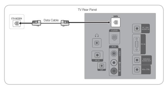
1. Connect the DATA jack of the TV to the [ETH MODEM] jack of the STB (SBB) with the Data cable.
