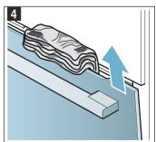
6. Push both retainers on the intermediate panel upwards, but do not remove it (figure 5). Hold the panel with one hand. Remove the panel.
