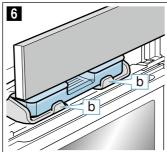
Slowly push the control panel downwards and then towards the rear until it is closed completely. The water tank has been filled. You can start operations with steam.
