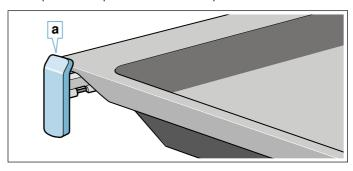
The pull-out rails lock in place when they are fully pulled out. This makes it easy to place the accessories in position. To unlock, push the pull-out rails back into the cooking compartment with a certain amount of force.
