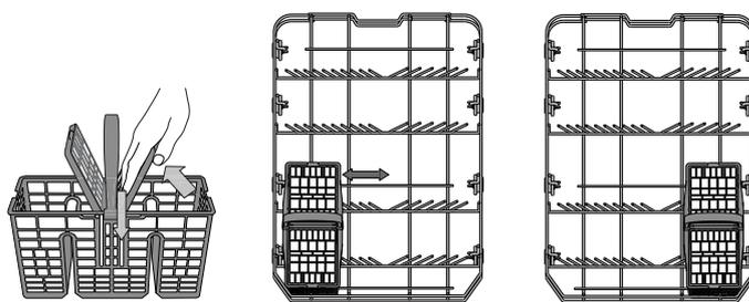
**Knives and other utensils with sharp edges must be placed in the cutlery basket with the points facing downwards or they must be positioned horizontally in the tip-up compartments on the upper rack.**
