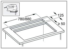
The angle between the cut surface and the worktop must be  $90^{\circ}$ .
