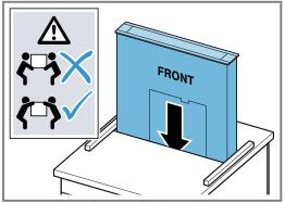
Insert the appliance evenly so that it is not tilted.4. Mark the cut-out for the pipework:
