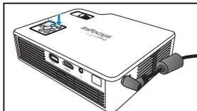
3. Press the Power button (⏻) to turn the projector on or off.
