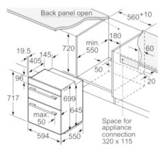
measurements in mm
