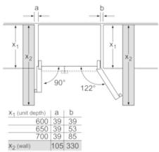
measurements in mm
