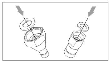
2. Install the two pads to the hose nuts.
