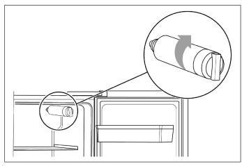
1. Screw in the new water filter in clockwise direction and make sure it is firmly fitted to the water filter base.
