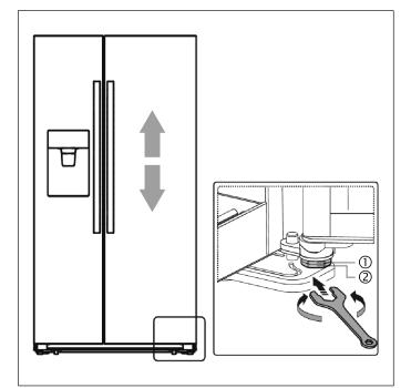
To raise the fridge door, turn the bolt (1) anticlockwise. To lower the fridge door, turn the bolt (1) clockwise. Once in position, lock the nut (2).
