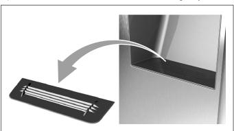
To clean the water collecting tray and the strainer, the strainer can be taken out.
