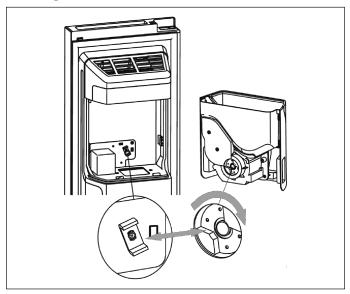
1. Check that the two couplers are at a suitable angle to connect correctly. If necessary, turn the coupler of the ice bucket to match the motor coupler.
