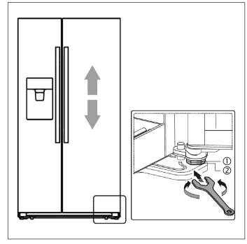
To raise the fridge door, turn the bolt (1) anticlockwise. To lower the fridge door, turn the bolt (1) clockwise. Once in position, lock the nut (2).
