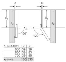
measurements in mm
