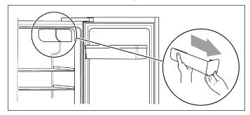
Open the refrigerator door to its maximum angle and remove the water filter cap by pulling it out slowly.
