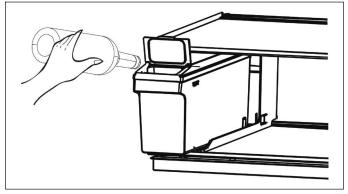
**2.** Lift the small front cover and pour in the water directly.
