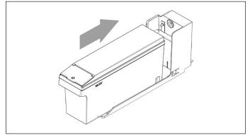
3. Refit the water storage box correctly.
