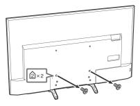
2 Attach the Wall-Mount Bracket (not supplied) using the screws (not supplied). KD-75/65/55XE90xx
