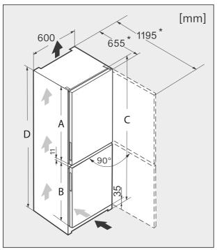
$<sup>^{\</sup>star}$  Dimensions without wall spacers fitted. Appliance depth is increased by 35 mm with the wall spacers supplied fitted.
