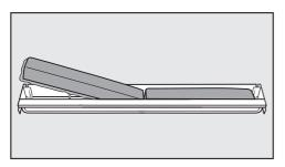
■ Remove both charcoal filters and place the new filters with the framed edge pointing downwards in the holder.
