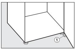
■ Ensure that you unscrew the adjustable foot ① from the lower hinge plate with the enclosed spanner until it sits on the floor. Then unscrew the foot by a further ¼ turn.
