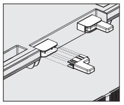
■ Fit the wall spacers onto the back of the appliance in between the transport handles.
