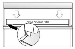
■ Place the holder in the middle of the raised edge at the back of the shelf, so that it clicks into position.
