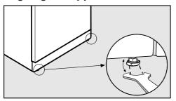
■ To align the appliance, adjust the front feet using the spanner supplied
