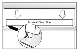
The charcoal filter holder clips onto the protective strip at the back of the shelf and can be moved as necessary.
