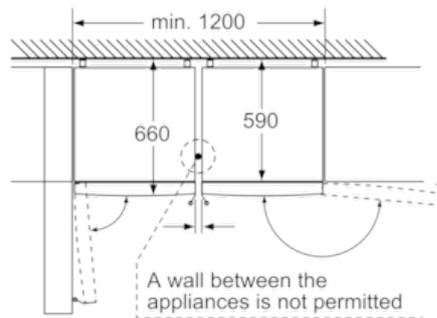
The two appliances shown are identical. (With different door hinges)
