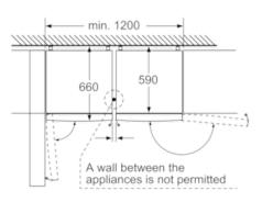
The two appliances shown are identical. (With different door hinges)
