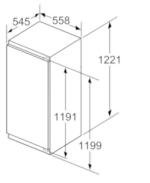
measurements in mm
