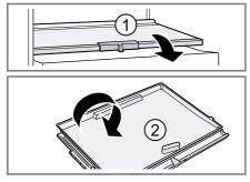
**3.** Press the fastenings for the lower glass plate outwards.
