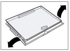
**4.** Lift the glass plate at the front ① and pull it out at the rear ②.
