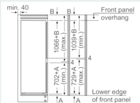
The specified unit door dimensions are valid for a door gap of 4 mm.
