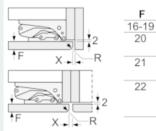
The gap dimensions recommended in the table must be adhered to in order to ensure that appliance doors do not collide with anything when they are opened, and to avoid causing damage to kitchen units.
