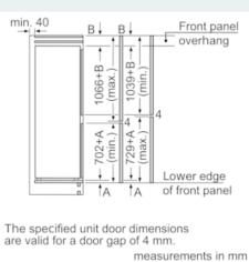
measurements in mm Recommended gap dimensions for flat hinges
