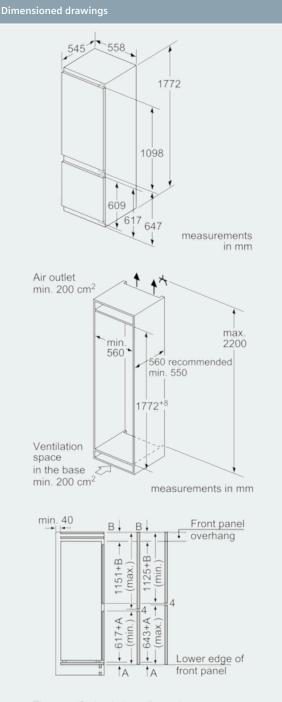
The specified unit door dimensions are valid for a door gap of 4 mm. measurements in mm measurements in mm Recommended gap dimensions for flat hinges
