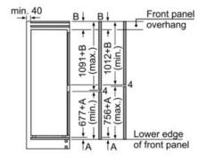
The specified unit door dimensions are valid for a door gap of 4 mm. measurements in mm
