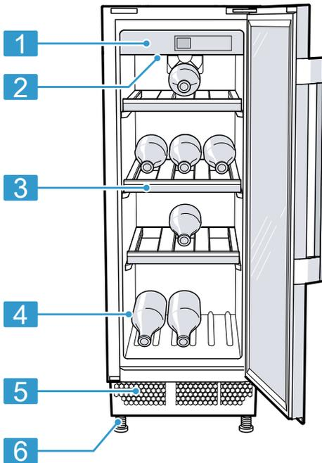
**1****1** Controls**2** Interior lighting**3** Bottle shelf**4** Rating plate**5** Ventilation grille**6** Screw foot
