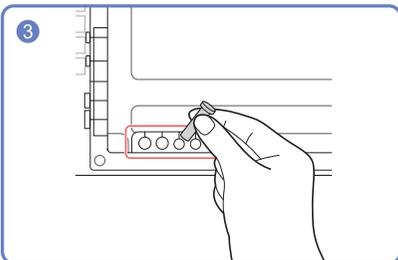
Insert and keep the removed Silicone-Bar in the marked area to ensure it is not lost.
