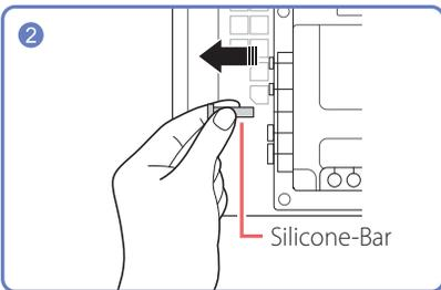
Remove the appropriate silicon bar for the thickness of the cable to connect.
