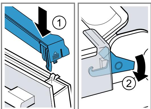
✓ The locking levers are closed. The appliance door is secured and cannot be detached.
