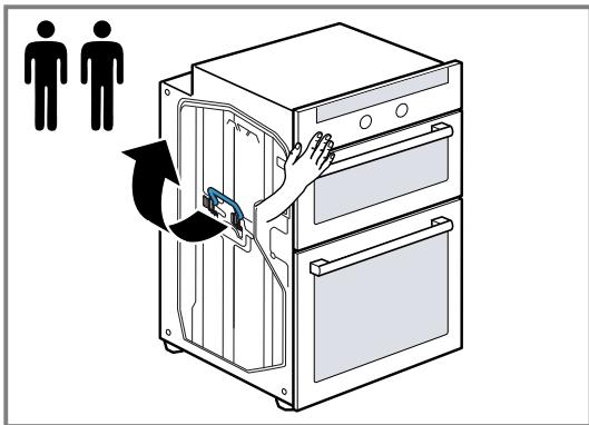
3. Place the appliance in the unit and fold the carry handles down.
