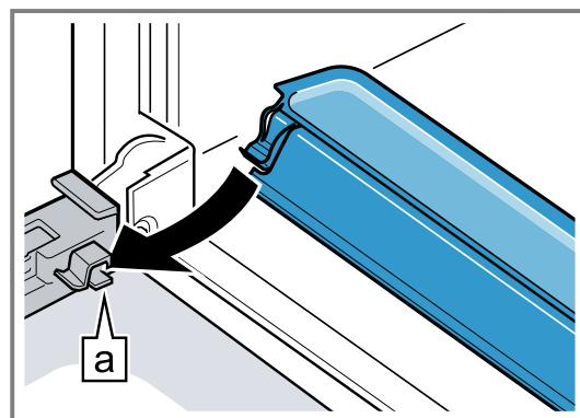
3. Slide the inner pane into the left- and right-hand retainers **a**.
