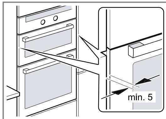
There must be an air gap of at least 5 mm between the appliance and adjacent unit fronts.
