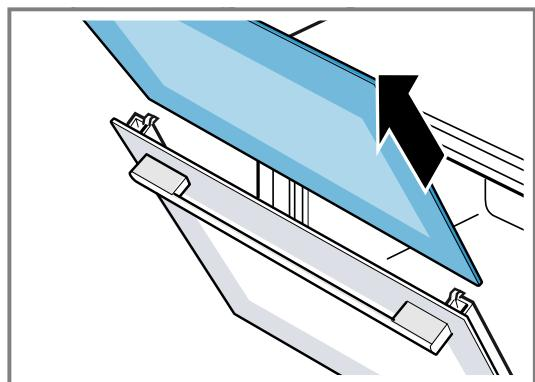
7. If necessary, you can remove the condensate trough for cleaning.
