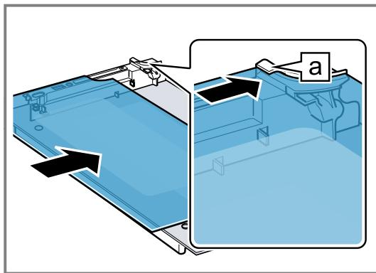
5. Push the inner pane upwards until it is in the left- and right-hand retainers **a**.
