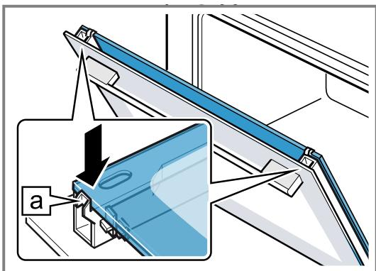
5. Put the door cover into position **①** and push down on it until you hear it click into place.
