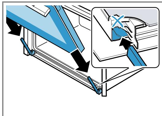
8. Close the locking levers on the left- and right-hand hinges.
