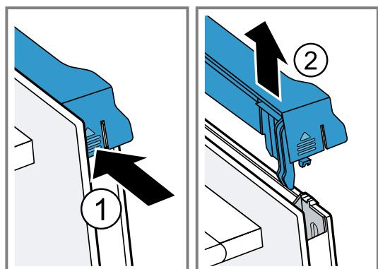
6. Lift out the inner pane ① and set it down carefully on a flat surface.
