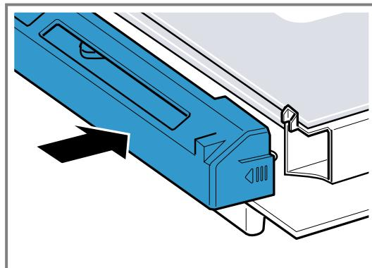
7. Slide the appliance door straight onto the two hinges. Slide the appliance door on as far as it will go. When doing so, ensure that the hinges are inserted into the correct opening.
