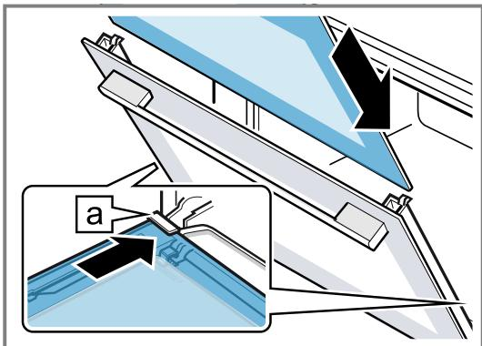
4. Push the inner pane upwards until it is in the left- and right-hand retainers **a**.
