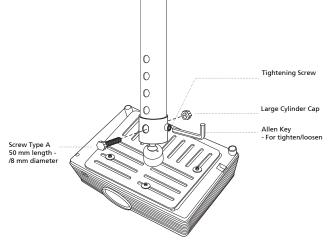
5 Adjust the angle and positioning as necessary.
