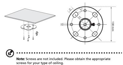
2 Secure the ceiling rod using the appropriate type of cylinder screws.
