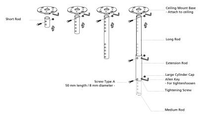
3 Use the appropriate number of screws for the projector size to attach the projector to the ceiling mount bracket.
