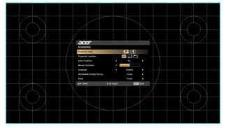
3 The background pattern acts as a guide to adjusting the calibration and alignment settings, such as screen size and distance, focus and more.
