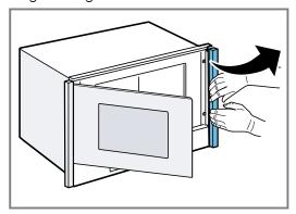
**4.** If the fastening elements have become loose when removing the panels, reattach them. Hook in the fastening element at the bottom and press down at the top until it is in place.
