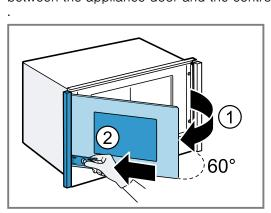
2. To loosen the panel, close the appliance door ① and at the same time press the fastening element on the appliance door down and towards the panel ②
