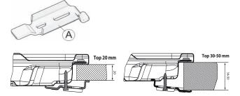
Where the hob is not installed over a built-in oven, a wooden panel must be installed as insulation. This must be placed at a minimum distance of 20 mm from the lower part of the hob.
