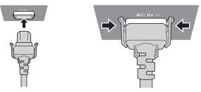
Check the shapes of the <AC IN> terminal on the rear of the projector body and the power cord connector, and insert the plug completely in the correct direction (until you hear the side tabs click in place).
