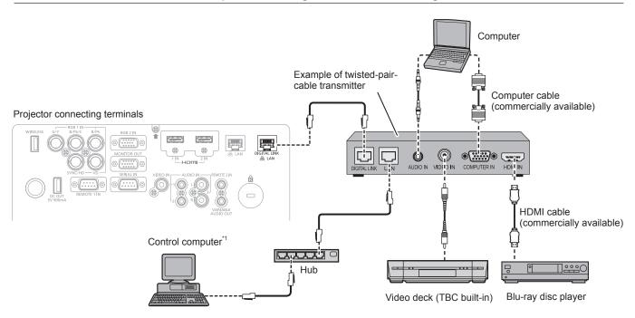
\*1 The control target will be the projector or the twisted-pair-cable transmitter. The control itself may not be possible depending on the twisted-paircable transmitter. Check the operating instructions of the device to be connected.
