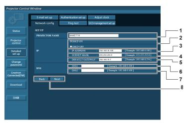
1 [PROJECTOR NAME] Enters the name of the projector. Enter the host name if it is required when using a DHCP server etc.
