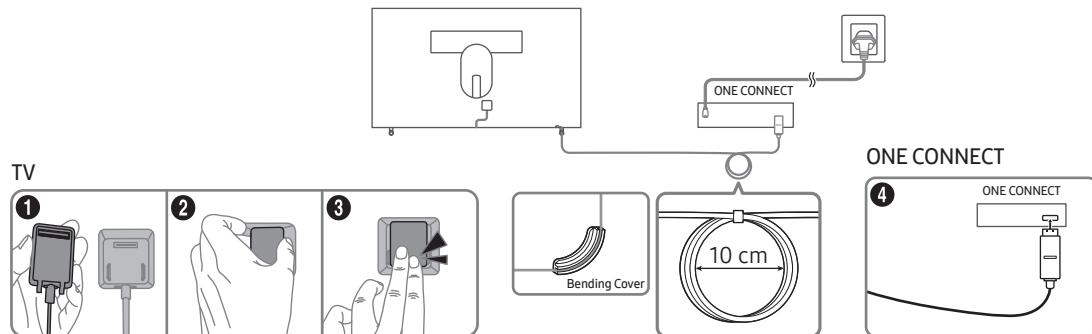
To connect the One Invisible Connection cable to the One Connect and your TV, take the following steps:
