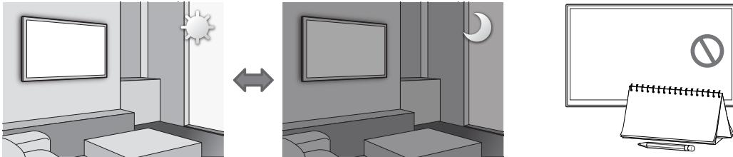
Eco Sensor adjusts the brightness of the TV automatically. This feature measures the light in your room and optimises the brightness of the TV automatically to reduce power consumption. If you want to turn this off, go to 🏠 > ⚙️ **Settings** > **General** > **Eco Solution** > **Ambient Light Detection**.
