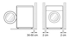
**Level floor** : Allowable slope under the entire appliance is  $1^{\circ}$ .
