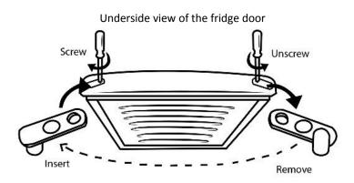
10. Place the fridge door back on to the middle hinge, put the pin of the top hinge into the top of the door and fix the hinge in to place by screwing it to the top of the fridge (use a spanner to tighten it if necessary). **Ensure the fridge door is aligned horizontally and vertically so that the seals are closed on all sides before finally tightening the top hinge.**
