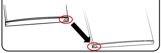
6. Tilt the appliance no more than 45 degrees and remove the right bottom hinge by removing the 3 screws with a cross headed screwdriver. Then remove the adjustable foot on the left side by unscrewing it by hand. Fix the bottom hinge to the left side with the screws and put the adjustable foot on the right hand side.
