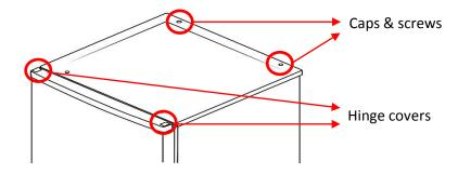
2. Remove the screws from the hinge bracket, take it off (you may need to twist the hinge before take the hinge away) and remove the fridge door by lifting it up and away.
