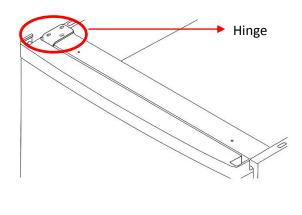
11. Replace the fridge door hinge covers, slide the top cover back and fix it in to place with the screws and replace the caps.
