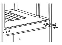
5. Remove the hinge plug from the bottom of the freezer door and move it to the opposite side and ensure it is fixed securely.
