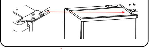
3. Remove the pin that is in the hinge with a screwdriver and flip over the hinge bracket before reattaching the pin to the hinge bracket. **Do not fix the hinge to the opposite side at this stage, please see step 10.**
