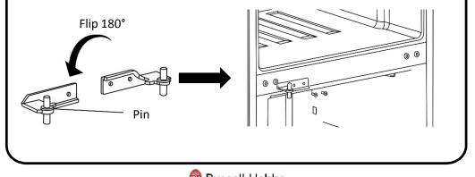
9. Remove the hinge adaptor from the bottom of the fridge door and fix the replacement hinge adaptor that is supplied as an accessory (packaged with the IB) to the opposite side, ensuring it is fixed securely.
