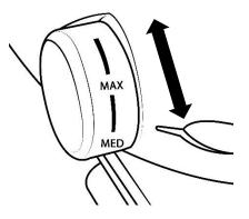
Depending on the ambient temperature of the room the appliance is situated in, you may need to adjust the temperature control dial; in a room with a high ambient temperature the temperature control dial may need to be adjusted to a colder setting (moved towards the MAX setting) or in a room with a low ambient temperature the temperature control dial may need to be adjusted to a warmer setting (moved towards the MED or MIN settings).
