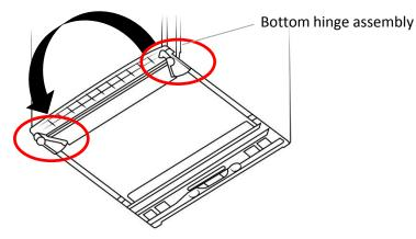
7. Place the freezer door on to the bottom hinge.
