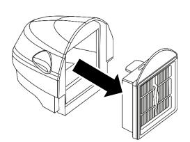
Remove the sponge filter from the HEPA filters To clean, remove excess dust from the filter using a soft brush. Wash in warm water and allow to dry for 24 hours.
