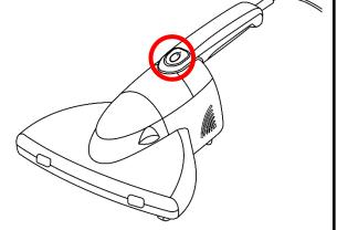
3. Ensure the two large wheels on the underside of the product are in contact with a flat surface, such as a mattress, then slowly move the vacuum cleaner back and forth over the surface.
