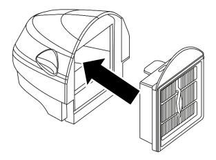
2. Insert the Dust Tank into the Vacuum Cleaner Unit.
