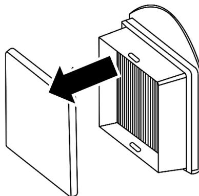
Once dry, replace the filters and the dust container into the vacuum cleaner unit.
