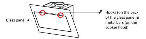
2. Gently lower the glass panel, ensure the latches on the cooker hood body at the bottom are open and carefully push the bottom of the glass panel towards the cooker hood. You should here a click and the panel should now be attached/locked to the cooker hood (ensure to check that the panel is attached to the cooker hood at the top and the bottom before letting go of the panel)
