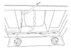
2. Unclip the light module from its terminal
