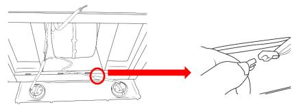
5. Replace the Aluminium grease filter and plug the appliance back into the mains or switch on the circuit breaker in the fuse box
