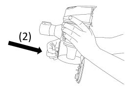
Once empty, close the bottom of the dust container then clip the dust container back into the vacuum cleaner unit, ensuring the bottom of the dust container is correctly located before the release button clicks back into place.
