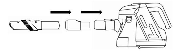
To use the brush tool, slide the brush to the end of the tool until it clicks into place.
