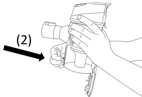
Once empty, close the bottom of the dust container then clip the dust container back into the vacuum cleaner unit, ensuring the bottom of the dust container is correctly located before the release button clicks back into place.
