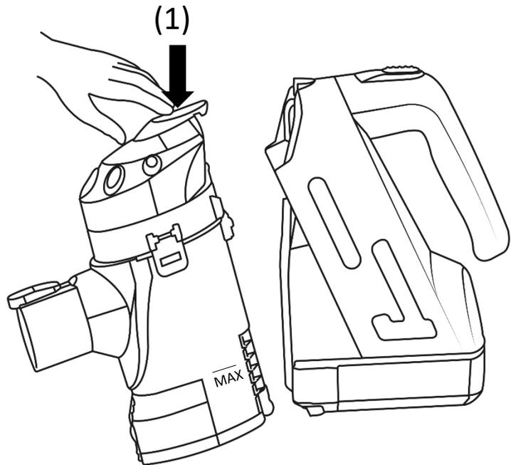
Whilst holding over a bin or inside a bin bag, press down the button on the dust container below the nozzle to open the bottom and release the dust (2).
