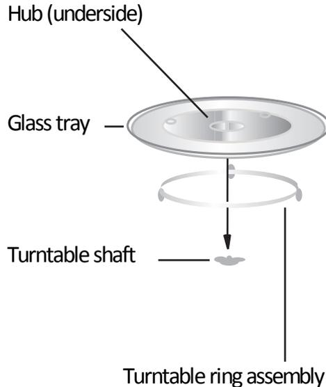
➤ Before first use, check that any securing tape has been removed from the glass tray and turntable ring assembly. These parts must never be restricted from rotating.
