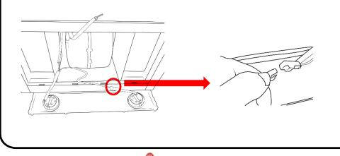
3. Remove the light from the its fitting in the front plate (this may require pressure or force to be applied).
