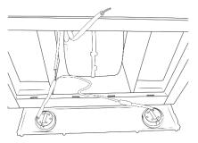
2. Unclip the light module from its terminal
