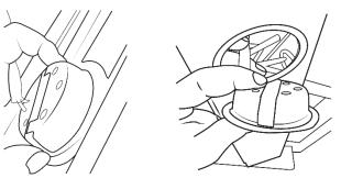
4. Put the replacement light module into the fitting (ensuring the terminal is threaded through the fitting) and connect it to the terminal.
