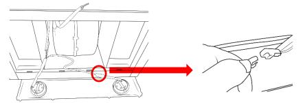
5. Replace the front panel (a cross headed screwdriver will be needed to fasten the screws into the front plate) and plug the appliance back into the mains or switch on the circuit breaker in the fuse box
