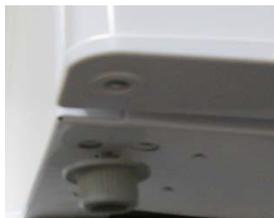
Remove the adjustable foot at the bottom of the fridge and set aside.
