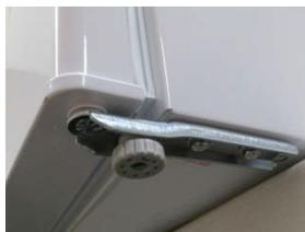
Unscrew the two screws holding the bottom door hinge and carefully moving it across to the opposite side and fix into position. Care must be taken as the door will be loose. Once this has been completed screw in the adjustable foot to the opposite side of the fridge.
