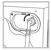
2. Connect the other end of the water inlet hose to the washing machine, screwing it onto the
