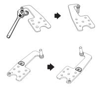
13. Reassemble the hinge on the refrigerator door by reversing the step 11.
