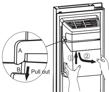
When you put it back, please make sure the two side (B&B') of Ice Bucket is wedged into the buckles (A&A').
