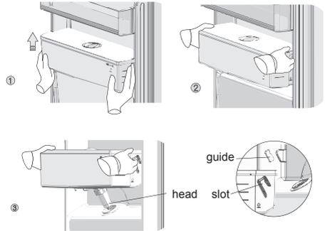
2. Hold the two sides of the water tank tightly, fit the water tank along the guides on the door.
