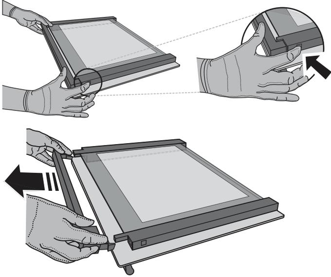
**2.** Lift and firmly hold the inner glass with both hands, remove it and place it on a soft surface before cleaning it.
