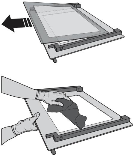
**3.** To correctly reposition the inner glass, make sure that the "R" is visible in the right-hand corner and the clear surface (not printed) is facing up. First insert the long side of the glass indicated by "R" into the support seats, then lower it into position. Refit the upper edge: A click will indicate correct positioning. Make sure the seal is secure before refitting the door.
