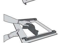
**3.** Refit the intermediate pane (marked with "R1") before refitting the inside pane: To position the panes of glass correctly, make sure that the "R" mark can be seen in the left-hand corner. First insert the long side of the glass indicated by "R" into the support seats, then lower it into position. Repeat this procedure for both panes of glass.
