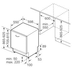
measurements in mm
